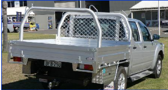
Alloy tray with optional removable rear ladder rack and underbody tool box
