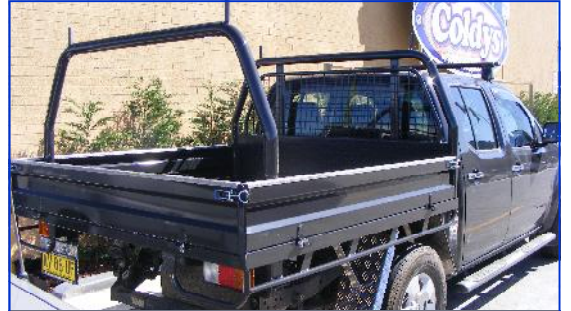
Heavy duty steel tray with optional removable rear ladder rack
