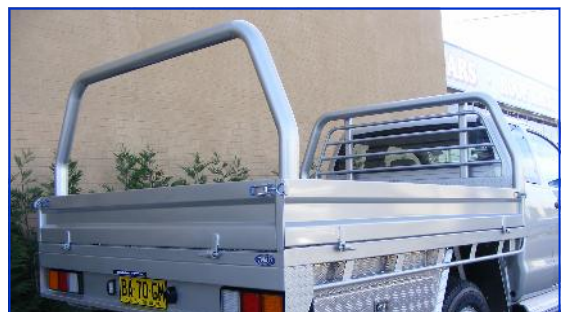
Alloy Tray with optional underbody toolbox and rear rack
