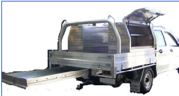
Alloy Tray with optional trundle tray and angled fixed toolbox
